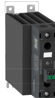
SSD1: 45 and 60 A single-phase SSR
